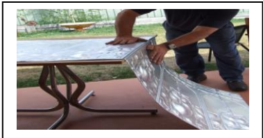
Showing how sheet can be folded simply Using a straight edge
