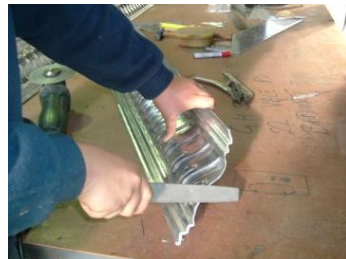
5/ De-burring of any sharp edges left on the cornice with a metal file.
