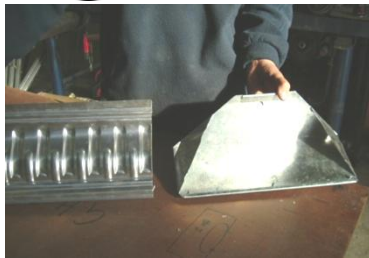
1/ Shows sliding the cornice into the mitre box for internal angle.
