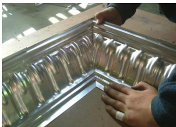
7/Picture shows both cornices coming together, just as they will be when installed.
