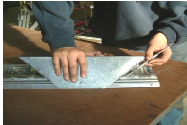
2/ Shows scribing in nominated position. Scriber to be held flat to end plate.
