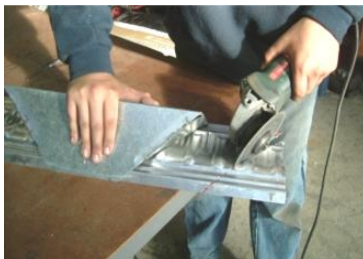
4/ Move back in mitre box until the scribed line is in line with the mitre box end plate. Now clamp and hold, remove the 5mm with cut off disc running on mitre box end plate.
